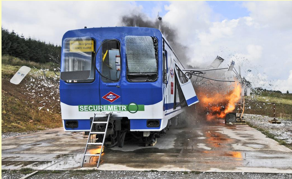
Blast testing a decommissioned metro vehicle.
