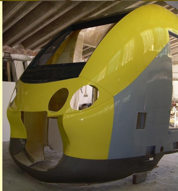
Lightweight crashworthy driver's cab - patented.
